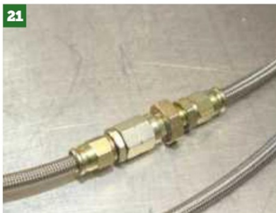
21 This is a bulkhead fitting, so you can fit the feed either side of the car's bulkhead, feeding into the bellhousing.
