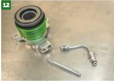
12 Dave prepares the slave cylinder next by removing the bleed and feed fittings — the former is replaced simply because it's not long enough in this application and is replaced.
