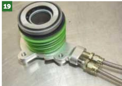
19 The system is pretty simple — this is the bleed fitting, which is cut so that the fitting sits outside of the aperture in the bellhousing, so you can get to it to bleed the system!
