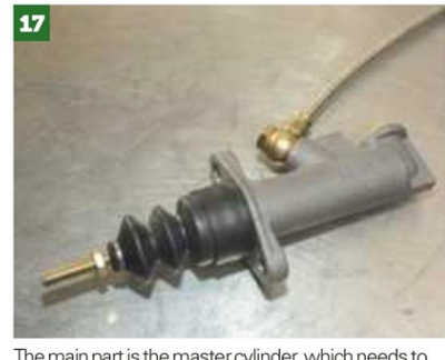
17 The main part is the master cylinder, which needs to be 5/8 inch. This is ideal for use with standard Ford pedal boxes with a fulcrum measurement of 55mm...
