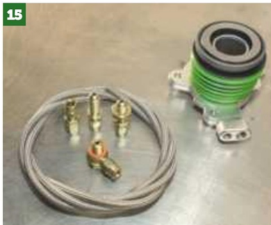
15 Sorting out the bleed and feed pipes is next. These are the components that come in the kit...
