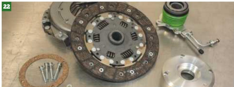
22 This system is meant to work with any engine application — Crossflow, Pinto or Zetec using a direct-replacement 215 mm clutch with a 1 inch, 23-spline centre on the Pinto and Zetec, and 190 mm clutch with a 1 inch, 23-spline on a Crossflow.
