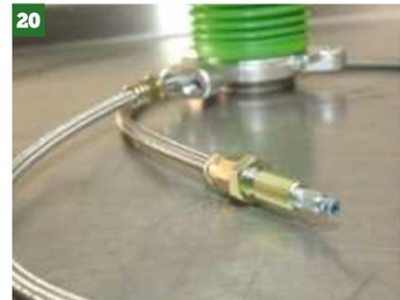
20 Back inside the bellhousing, you can see the orientation of the braided hoses, connecting with the fittings in the plate.
