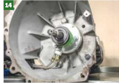
14 Fitted, you can see the pipes need to sit opposite the opening in the bellhousing — this is a special cut-away piece that Dave's prepared so we can see the slave cylinder mounted later on.
