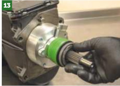
13 The slave cylinder can be fitted now, but there are four positions it can be orientated to — although you can't see this without the bellhousing in place!
