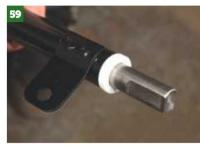
...Which has a corresponding flat on one side, forming the D-shape.
