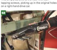
The last bit is the steering column shroud, which picks up on the original column mounts..
