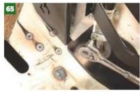
Once that lot's bolted up, Dave then finally tightens the universal joint fixing at the bottom of the column.
