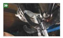
Then they bolt up onto the underside of the strut using supplied fixings - although they will probably need some assistance from a jack as the anti-roll bar is spring-loaded, of course.
