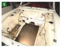
This stripped-out shell is ready for the kit to be bolted in. This is an early left-hand-drive shell that's been converted to right-hand-drive
