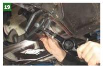
Dave slides these into the crossmember and slots the new bolt through, which is locked up with a Nyloc nut.
