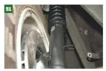
Generally, the 2.8i discs will bind on the coil spring if you run 2.25 inch coil-overs, meaning you need to use the wider Retro Ford alloy hubs.
