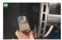
It is easy to get the steering arms on the wrong way round, but you'll know because the gap between disc and steering arm eye is massive.
