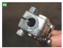
The splined end goes onto the rack...
