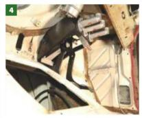
Under the dash is a Retro Ford bias pedal box, ready-fitted, which bolts straight in.
