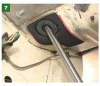
Once installed in the new pressing, there's a hole for the steering column shaft to pass through.
