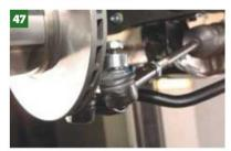
...These are very close to the disc if you have vented discs fitted — done to create the all-important, correct Ackermann angle.
