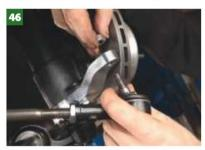
The track rod ends are then bolted into the steering arms although, again we need to point out that...
