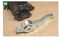
Adapting them into the car are Retro Forddesigned and CNC-fabricated, steel billet bottom steering arms. These are handed.
