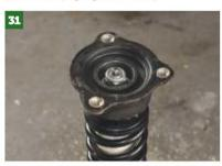
The struts will be bolted into the shell using standard Cortina roller top mounts.
