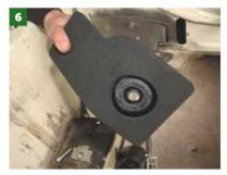
The new hole's blocked up with this cover plate, which fits from inside the car and additionally carries foam insulation.
