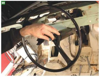
.. Followed by the steering wheel. All done! This is a right-hand-drive Pre-Aeroflow car which has a slightly longer column, but Dave can supply kits for the later Aeroflow, as well as left-hand-drive cars, too. CF
