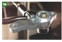
They bolt onto the end of the TCA first, using a supplied Nyloc nut. This will sit inside the assembly and can't be seen once the strut's fitted.
