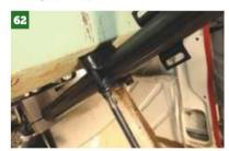
Again, it's engineered to use the original fixings built into the car — this Cortina clamp fits around the column and fixes to the underside of the dash...
