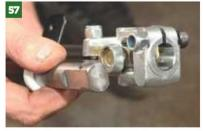
Moving to the other end of the shaft, there are two of the same type fittings on another universal joint — Double-Ds.
