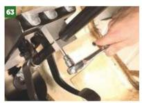
..Then to the alloy block that forms the secondary fixing if you're using the Retro Ford bias pedal box.
