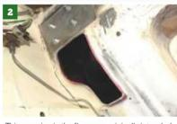
This pressing in the floor was originally intended for the steering box to pass through. The pressing is identical left and right — it's a simple matter off cutting it open when swapping the steering from left to right...
