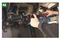
**Steering Rack** The next job is to prepare the rack for loading it into the crossmember.
