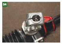
...While the Double D end connects with the shaft — this needs setting up.
