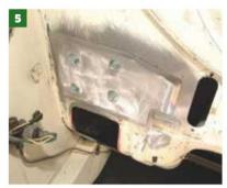
Although Dave's added additional strength to the area, as it can flex under extreme braking!
