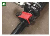
The rack's fitted with normal saddle clamps and poly bushes; again supplied.
