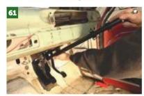
The column can then be fitted onto it from inside the car — loosely for now. Grease the shaft where it passes through the grommet.
