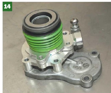
14 ...The Retro Ford concentric release bearing to be bolted to the front.
