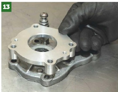
13 Next bit is this billet aluminium adapter plate, which corresponds with the Mazda mounting bolt holes allowing...
