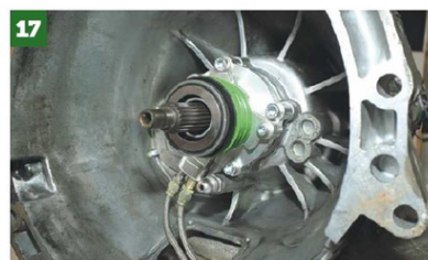
17 Once it's bolted in place, you can see that the feed pipes are orientated towards one of the access holes in the bellhousing — the feed pipe and the bleed tube are replaced with remote units. Retro Ford uses braided hose and for now, the pipes exit through the original release arm hole.
