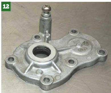
12 The guide tube can then be simply cut off with a hacksaw and dressed with a file.
