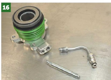
16 The release bearing is next but it needs some adaption first. It comes supplied with a feed pipe and an extended bleed screw — both of these need removing.
