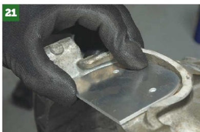
21 Finally in this section, there is another hole in the bellhousing, which needs filling over this is was the starter motor hole in the MX5 application — Retro Ford supplies another alloy plate, which is simply bolted in place.
