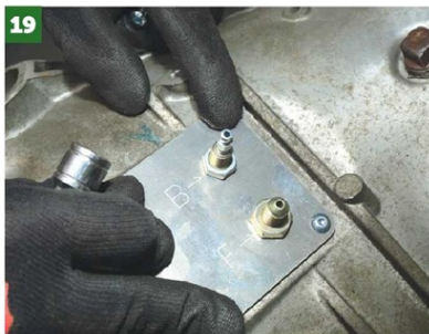
19 ...To accept this alloy plate, which has two fittings attached. One is for bleed, the other for feed, which is clearly etched into the plate's face.
