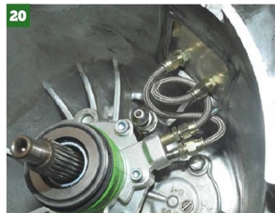
20 Back inside the bellhousing, you can see the orientation of the braided hoses, connecting with the fittings in the plate.
