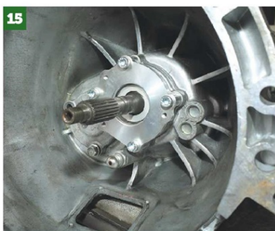
15 The adapter plate goes into the bellhousing, bolting to the front of the gearbox face.
