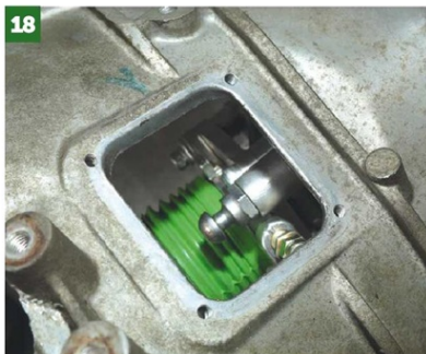
18 This is the view through the access hole — you can see the outer edges have been drilled and tapped...
