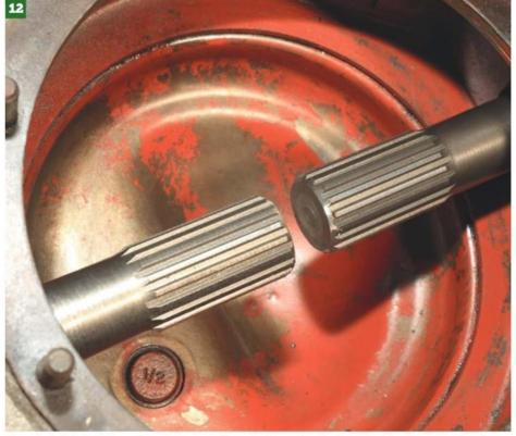
Once the halfshafts fit the casing, you can see with a pair of Escort-length shafts fitted that the centres virtually touch. This gap is the part Dave works out—also taking into account that an LSD will usually have a thicker centre crosspin which isn't always allowed for with all aftermarket halfshafts. Believe it or not, they can be too long and bottom out on the pin. This bit is critical and Retro Ford pays particular attention to it meaning their shafts fit!
