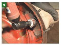
Therefore, it will need dressing back for which Dave uses a rotary sander in an air tool. The casing will need to be cleaned out afterwards to avoid getting damaging swarf in the bearings and differential unit.
