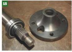
...and the end flange slides off another spline on the end of the halfshaft, which means the shafts can be supplied in various lengths, the end flange slid on and the whole lot still retains its strength.
