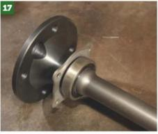
This is deliberate because it appears that the bearing is running the wrong way round with oil seal facing out. For technical reasons, this is necessary.
