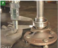
By contrast, the bearings on an Escort — and indeed Mk2 Cortina — are 22 mm thick.
