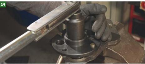
Undo the centre nut, which is shown here being torqued up...
