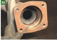
This is a small bearing case from a Mk1 Cortina saloon, which also has this oil seal. These can be left in the casing, which the larger bearing cases don't have they use a seal around the bearing.
