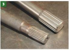
...although the main difference is in the spline count and size. Standard is 22-spline, and above it is the 18-spline that Retro Ford's Cortina-size halfshafts are made to — and there's a reason!
