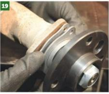
Here you can see where the ring fits in front of the oil seal retainer. The whole lot is designed with care so that you don't upset the offset of the wheels either.
