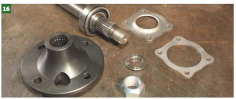
There are a couple more components of the halfshaft system that need explaining here — at the top, there's a pressed plate with a dome in it, and this retains the bearing.
