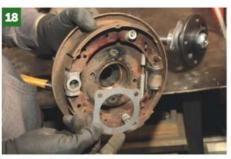
The other plate is used in place of the drum backplate. If you're still retaining drums, then you don't need this bit but if you convert to discs, then this spacing ring takes the place of the backplate — leave it out and you could upset and distort the keeper plate. It's a small thing, but it's the details that matter!
