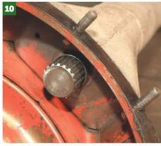
Once it's opened up, the halfshaft will easily pass right through the casing.
