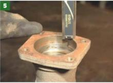
Apart from the width of the casing, there are differences in bearing size in the ends — with a pair of vemier callipers, you can measure the depth. This is a Mk1 Cortina casing...
