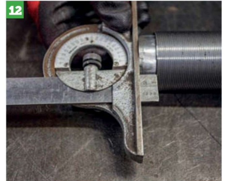
The sleeve needs to be positioned 15 mm from the top of the tube.
