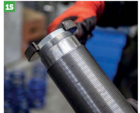
Before you fit the new insert, carefully test fit the new retaining nut to make sure it threads onto the tube properly.
