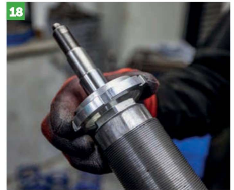
Now thread on the bottom collar, making sure the shoulder is pointing upwards...
